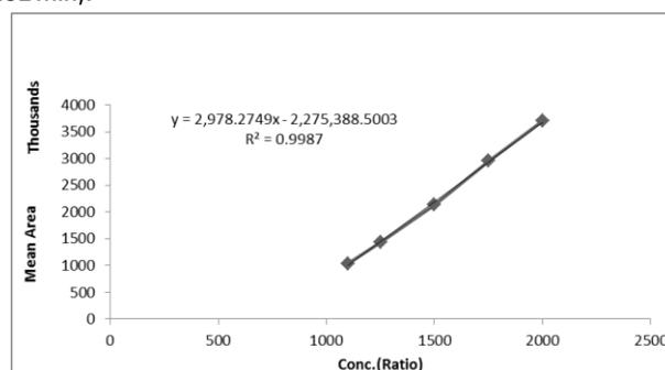
Figure 2. Calibration curve of standard artemether
