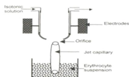
**Figure 6:** Electro encapsulation technique
