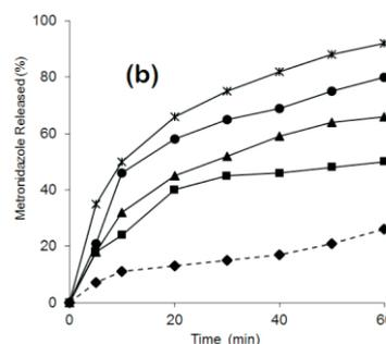
**Figure 2(b):** Dissolution profiles of metronidazole tablets formulated with different concentrations (%w/w) of MCC extracted with sodium hydroxide. 0 (♦), 2.5 (■), 5 (▲), 7.5 (●), 10 (✱)
