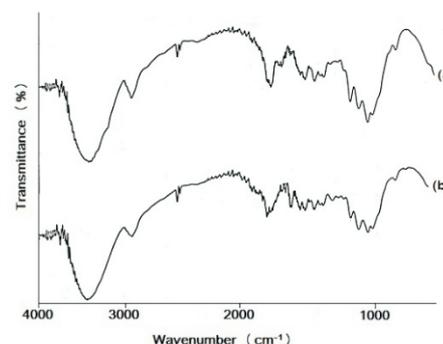
**Figure 1:** FTIR spectra of the extracted microcrystalline cellulose powders using nitric acid (a) and sodium hydroxide (b) as extracting solvent
