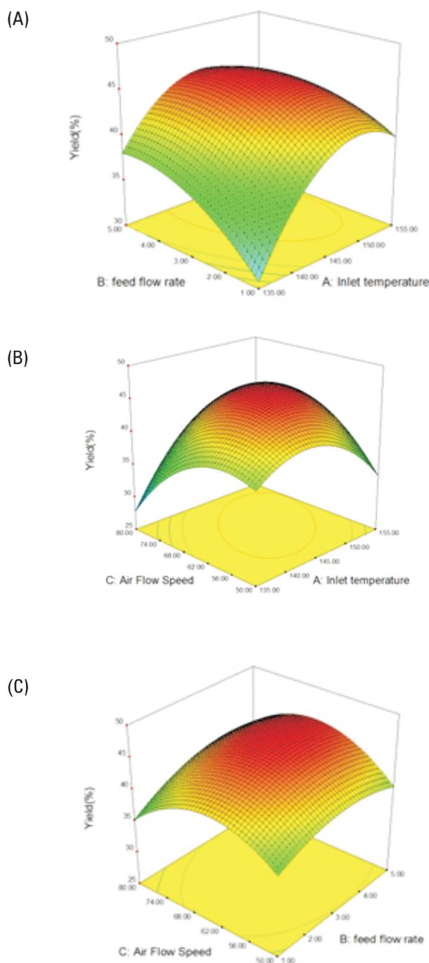
**Figure 2:** Response surface plots for product yield. (A) inlet temperature, (B) feed flow rate, (C) air flow speed
