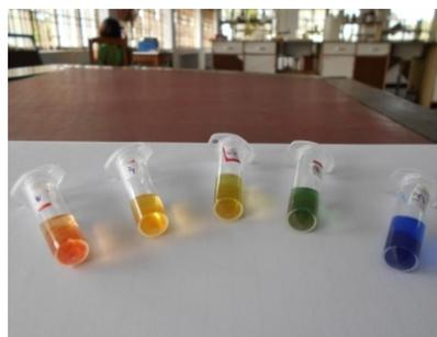
**Figure 3:** Hydrogels smartly changing color at different pH values (pH 1.0, pH 4.0, pH 6.0, pH 8.0 and pH 10.0, respectively).
