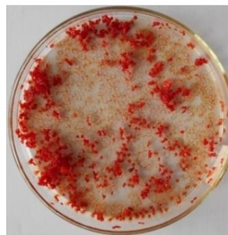
**Figure 2.** Bromothymol blue entrapped gellan gum hydrogel beads
